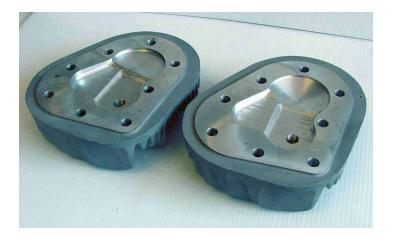
**WR** machined to the factory 49 R drawing Volume 65cc
