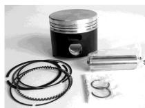
Manufactured for us by **WISECO**, these are the highest quality forged pistons available. 1 mm top ring, 1.2 mm second ring and 3 piece oil ring,. Coated skirt, complete with pin and wire locks.
